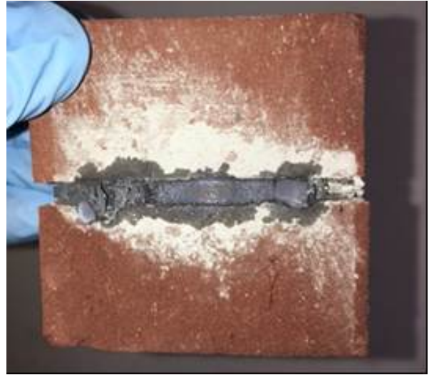
Fig. 2. Two ceramic tiles made of JSC-1A lunar regolith simulant and joined by combustion of aluminum/nickel mixture placed between them and ignited with a laser.
